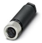
Connector, 3-position, Socket straight M8, A-coded, Screw connection, knurl material: Nickel-plated brass, external cable diameter 3.5 mm ... 5 mm
